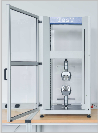
Materials testing machines for tensile, compressive and bending testing
