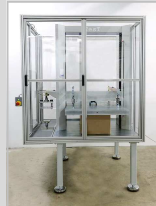
Testing machine for package materials (BCT)
